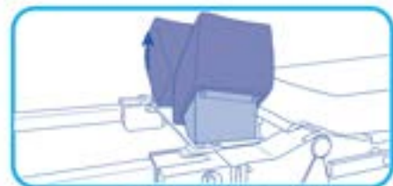
3 Caution: to remove the supports, only pull them straight upwards to avoid damaging the fastening mechanisms.
