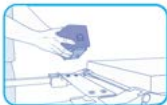
1 First place one and then the other thigh support on the adaptor.
