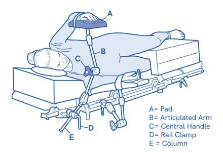
**CS Universal Arm Support-**Extended; used to position the patients arm in the prone, supine or lateral position.
