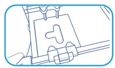
Snap the locking clip shut to secure the attachement in position.
