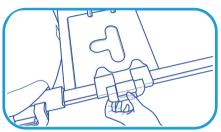
Place the attachment on the frame so that the brackets are over the bars.
