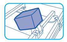
Snap the locking clip shut to secure the support in position
