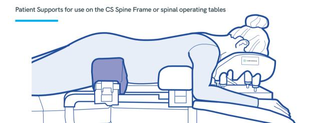
Refer to the label on the support to ensure it is placed in the correct position on the table.
