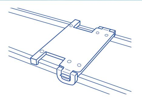
The CS Supine Top (Base Only) can be attached to most dual-rail operating tables on the market\*
