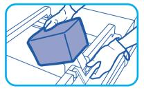
Place the supports on the frame so that the brackets are over the bars
