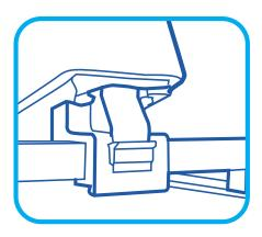
Push the clip down to lock the support securely in position.
