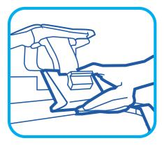
Place the chest and hip supports on the frame as shown so that the brackets are over the frame.
