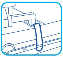
Tighten the straps until the frame is firmly attached to the table to prevent movement during the procedure.
