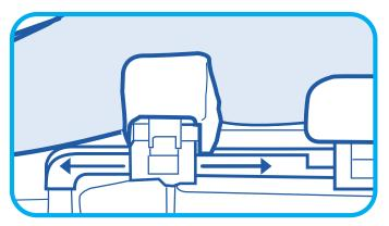
To adjust the position of the supports, release the clip(s), raise the patients chest or hips, slide the supports to the correct position, re-fasten the clip(s).
