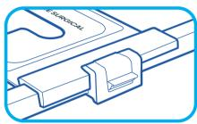
Snap the locking clip shut to secure the attachment in position
