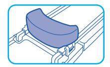
Snap the locking clip shut to secure the support in position
