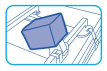
Snap the locking clip shut to 2 secure the support in position
