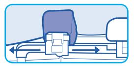
To adjust the position of the supports, release the 3 clip(s), raise the patient's chest or hips, slide the supports to the correct position, lock the clip(s)
